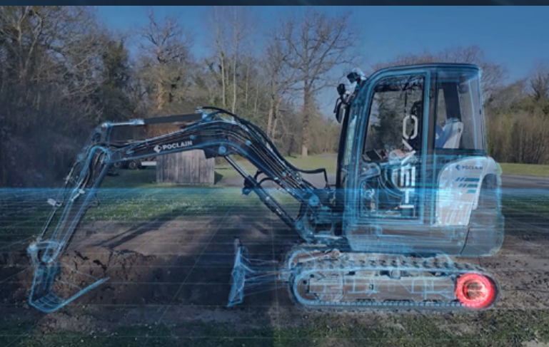
Mini excavator equipped with a HEVO-BOOSTER to boost the pressure of the motors in the tracks
