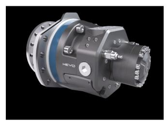
The Hevo Booster range is designed for wheel-type applications that experience high torque peaks and require limited speed. The concept is straightforward: the motor operates on a small nominal displacement sufficient for more than 90% of its usage time. When torque peaks occur, an internal pressure booster activates, potentially doubling the pressure inside the main cylinder block up to 800 bars for a short duration.
