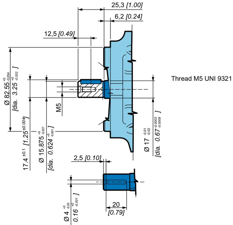
**D2** Ø 18 [dia. 0.71]; Max. torque: 100 N.m [885 in.lbf]
